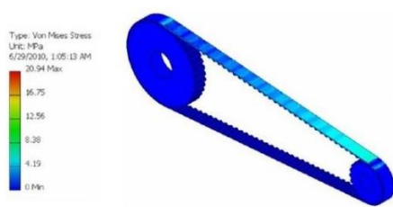
Figure 17 Von-mises stress at M = 7.5 N-m.
