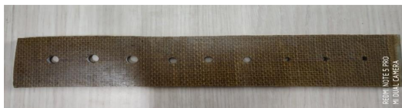
Figure 5 The sample specimen with the drilled holes.
