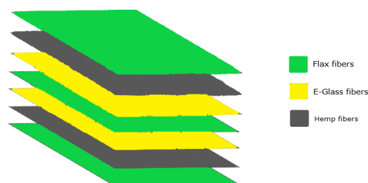
Figure 1 Stacking order of reinforcement fibres.
