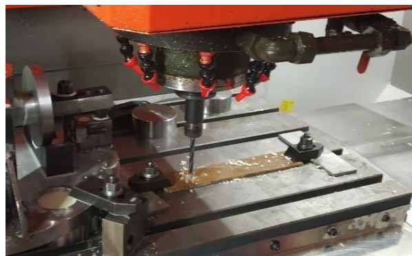
Figure 2 Experimental set-up with vertical machining centre and drill bit
