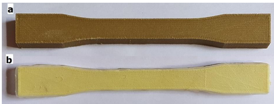
Figure 5 (a) Uncoated and (b) Coated tensile specimens.
