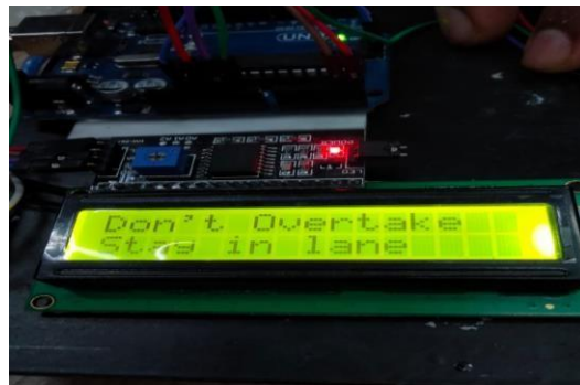
Figure 12 Data to be displayed in the vehicle.
