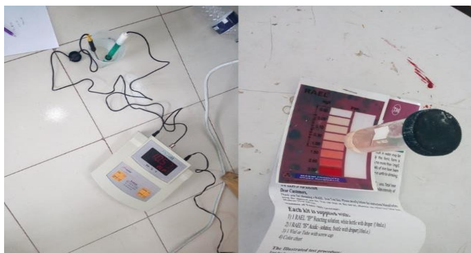
Figure 13 pH, temperature, and iron concentration test.
