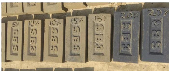
Figure 2 Bricks with different % of rice husk ash.
