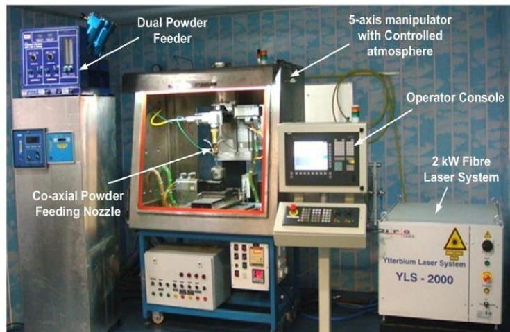
Figure 2 Direct energy deposition apparatus (Courtesy: RRCAT, Indore, MP, India).
