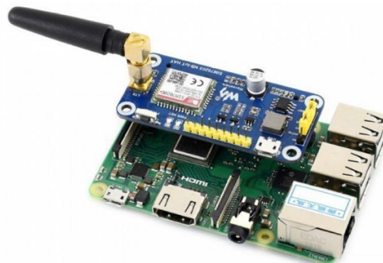
Figure 3 Raspberry Pi 2 model B with SIM7020E NB-IoT HAT module.
